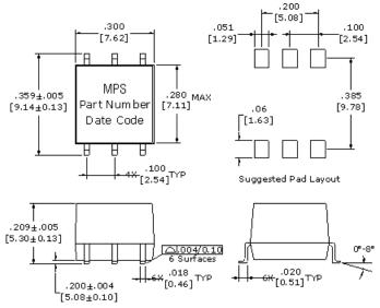
Dimensions: in/mm. Tolerance:  $\pm$ .010/0.25 unless otherwise specified.
